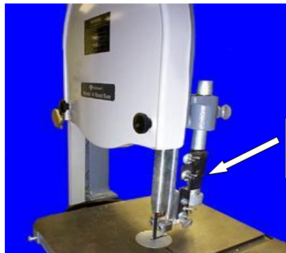
Bandsaw blade adjustable guard
