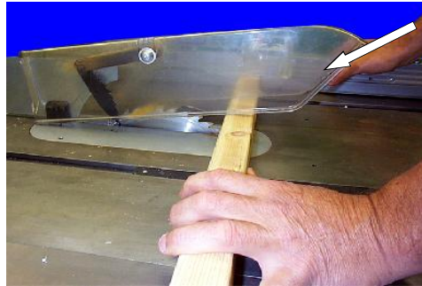
Circular table saw self-adjusting guard
